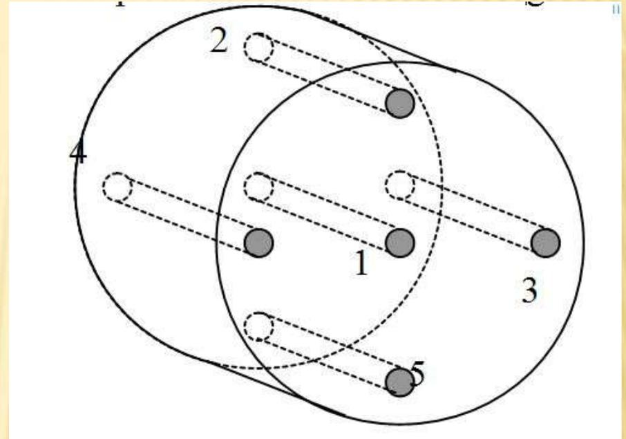
PMMA phantom for measurement of CTDI
