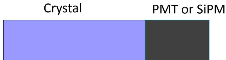
Scintillator based radiation detector.
