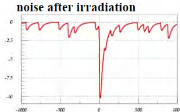
Strips, fibers, glue etc do not degrade at estimated radiation dose
