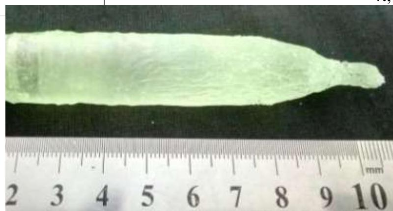
Light output of YAGG:Ce,C = 300 % BGO = 125% YAGG:Ce (~40000 phot/MeV)
