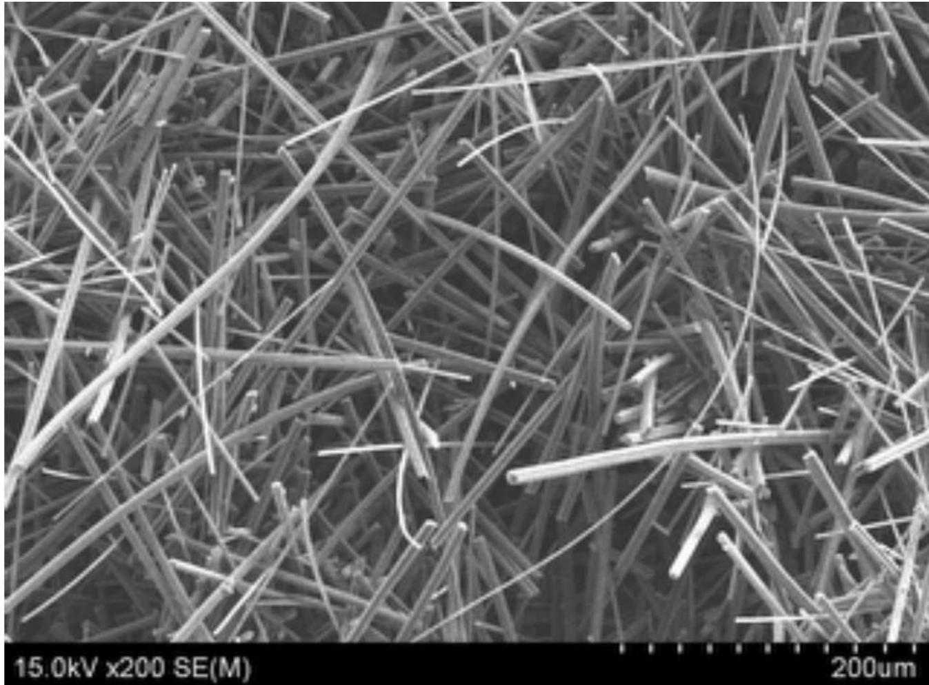
**Carbon fibers** or graphite fibers are fibers about 5–10 micrometers in diameter and composed mostly of carbon atoms. Carbon fibers have several advantages including high stiffness, high tensile strength, low weight, high chemical resistance, high temperature tolerance and low thermal expansion.
