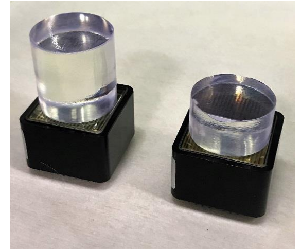
ScintiClear sensors on R11265U PMTs before and after encapsulation.
