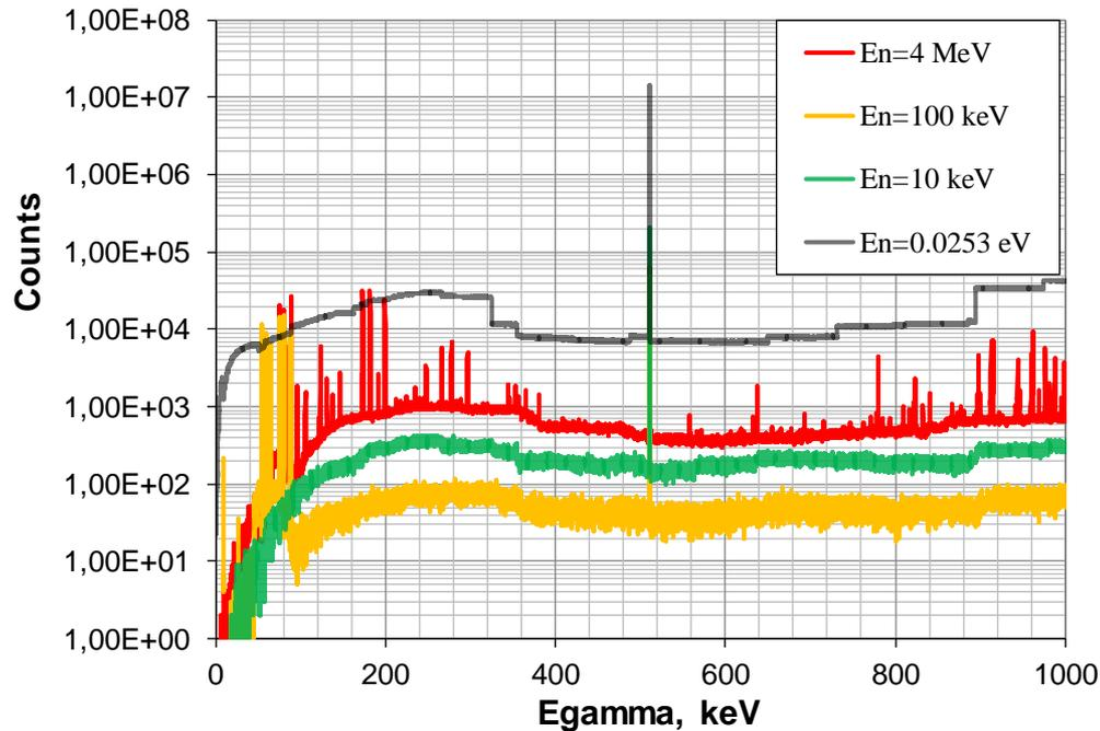
Spectra of the emitted gamma-quanta in metallic gadolinium with 2 mm thickness, irradiated with monochromatic neutrons in a broad energy range, simulated with GEANT4.
