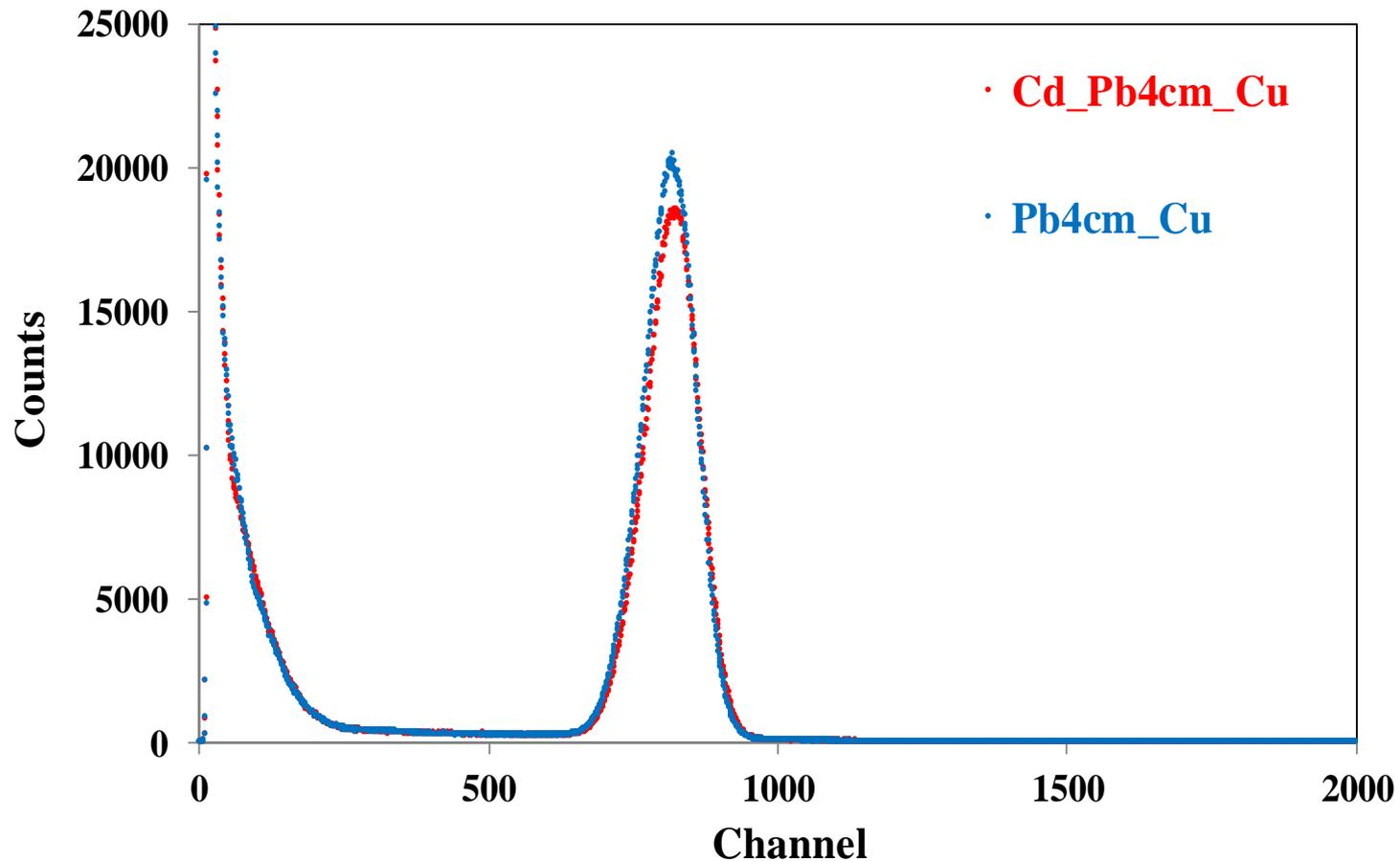
**Comparison of countrates measured with  $^6\text{Li}$  KGS glass ceramics (neutron peak) and GAGG: Ce,Mg,Ti crystal (90, 190, 511 keV lines) in the same position relative to Am-Be source.**
