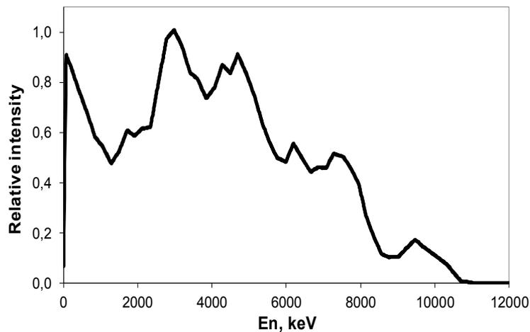
Spectrum of neutron energies from Am-Be neutron source, in accordance with ISO 8529-1:2001(E)
