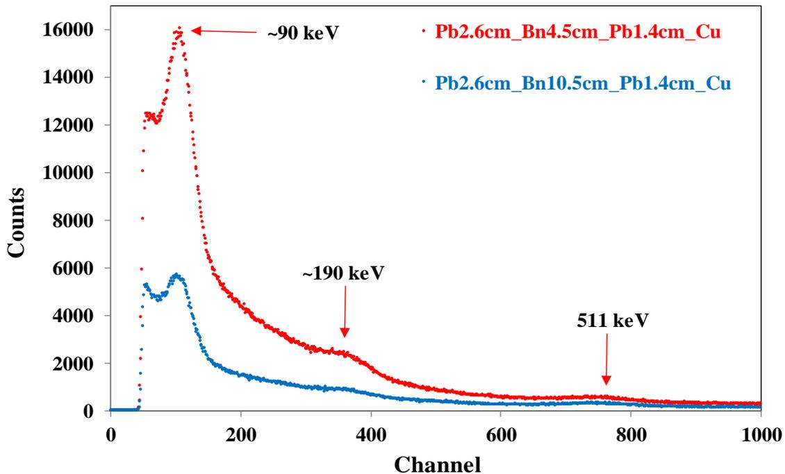
Increase of the boron acid absorber thickness from 4.5 cm to 10.5 cm transforms neutron source spectrum, which results in a decrease of the area of ~90 keV line in more than 4 times, while the area of 511 keV line decreases only by a factor of 2.
