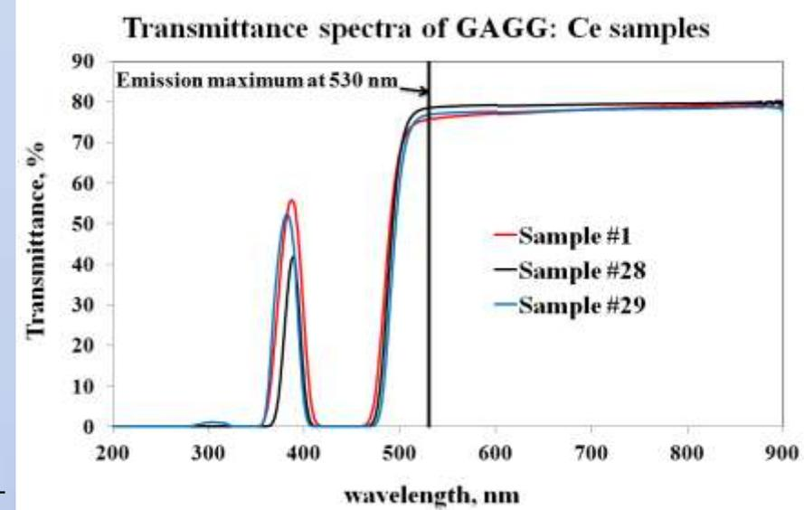
$$\Delta k = \ln \left( \frac{T_{bef}}{T_{after}} \right) \cdot \frac{1}{d}$$
