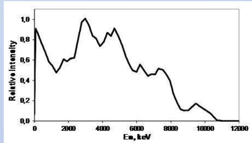
Spectrum of neutron energies from Am-Be neutron source, in accordance with ISO 8529-1:2001(E)
