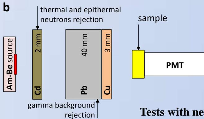
Kozlov D. Setup for characterization of scintillators to detect neutrons
