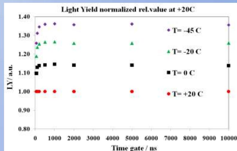
Light Yield vs integration time was measured (Hamamatsu PMT XP 2059,  $^{241}\text{Am}$ )
