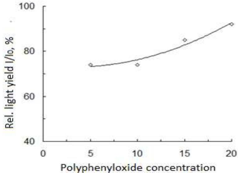
The introduction of diffusion amplifiers into the polymer base of a PS can lead to an increase in its radiation hardness.
