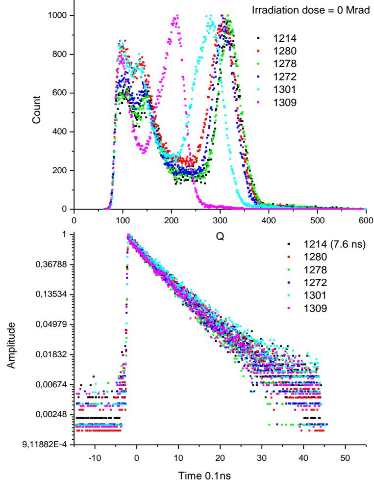
Under of irradiation, degradation occurs not only in the polymer base but also in the activator molecules. It is generally known that fluorination leads to an increase in the photostability of dye molecules.
