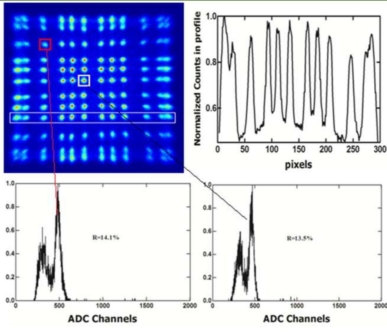
Top: Raw image of the 12x12 GAGG:Ce scintillator array and a horizontal line profile of the scintillator elements under  $^{137}\text{Cs}$  excitation;
