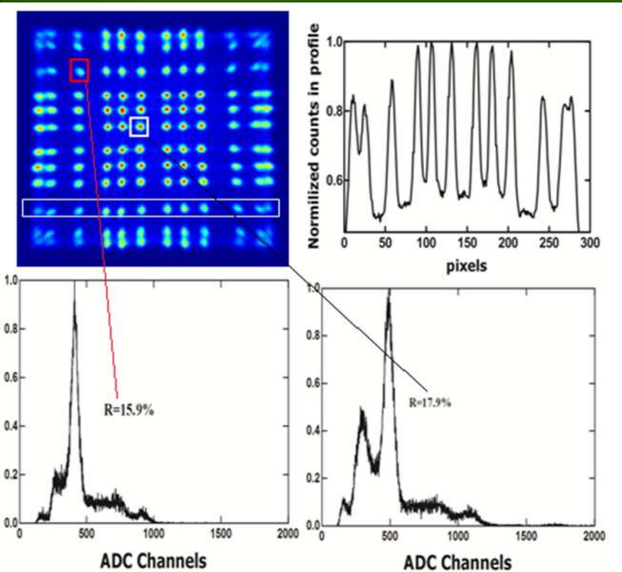
Top: Raw image of the 12x12 GAGG:Ce scintillator array and a horizontal line profile of the scintillator elements under  $^{22}\text{Na}$  excitation;
