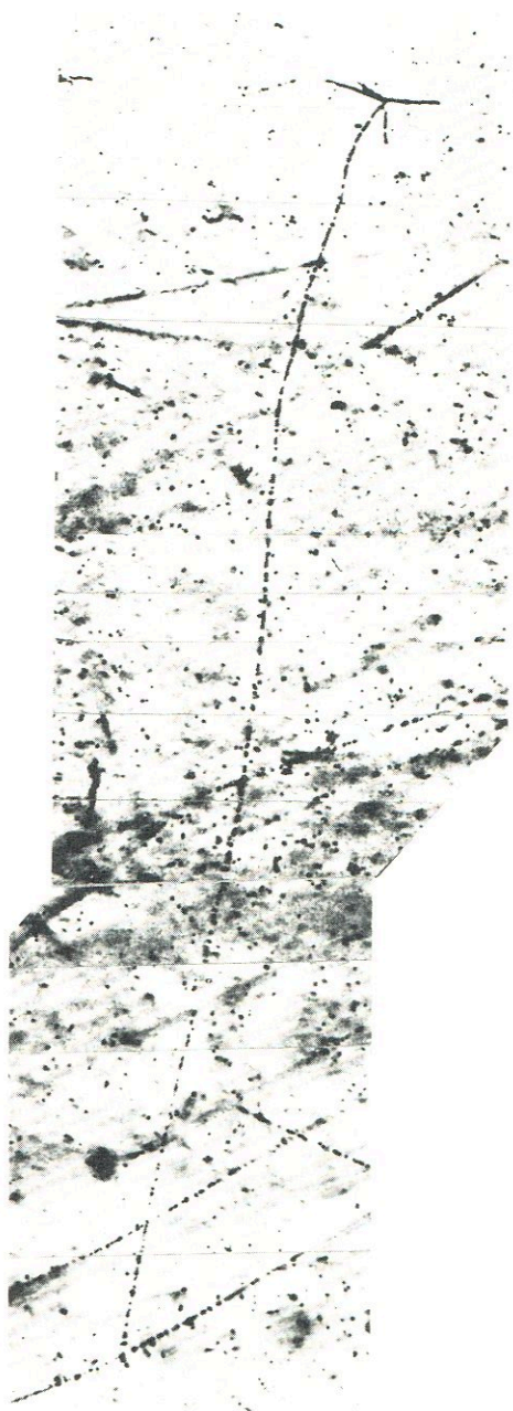
FIG. 1.1.1. Photomicrograph of a negative \pi meson track produced in C-2 emulsion during the course of the experiment leading to the first artificial production of \pi mesons. (Photomicrograph by A. Oliver.)
