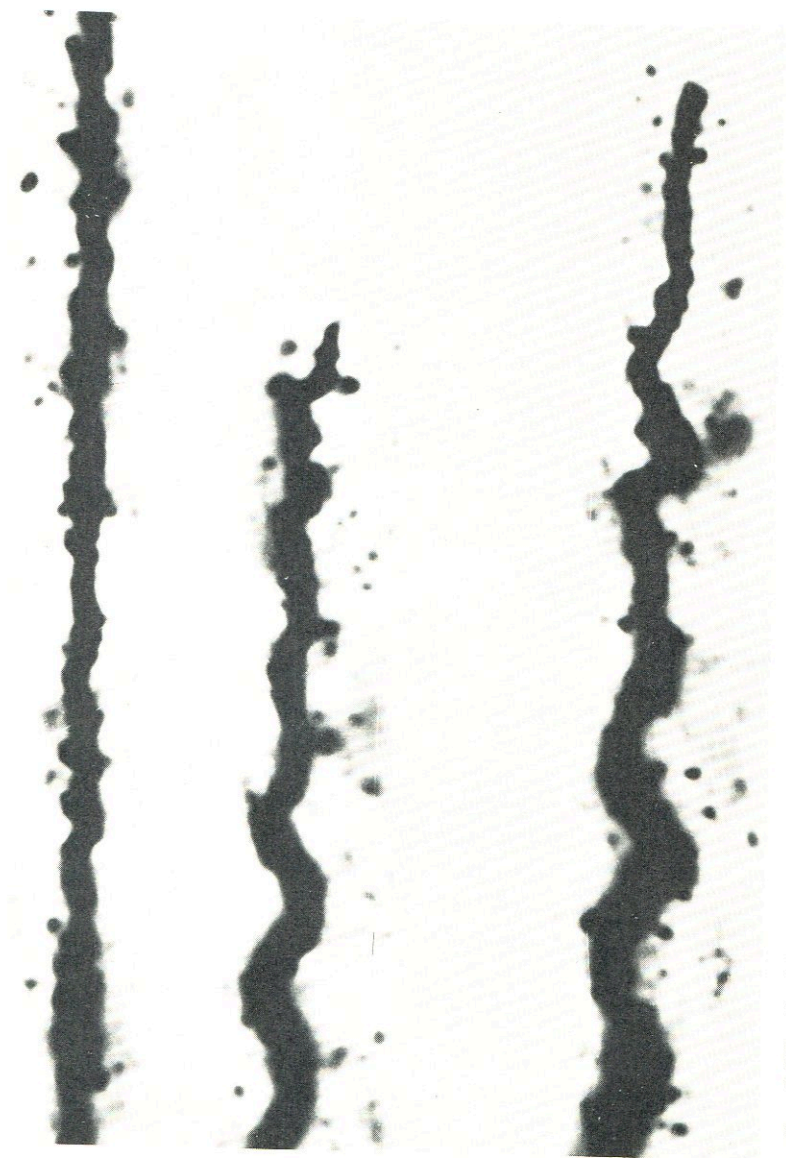
FIG. 2.3.1. Buckled tracks of two A^{10} ions, and also the track of an N^{14} ion in G.5 emulsion. They show the effect of physical development on tracks of very highly ionizing particles. Argon ions in the buckled region suffer energy loss at a rate of about 5 Mev/ \mu . The nitrogen track is only slightly buckled although its rate of energy loss is about 1 Mev/ \mu . (Photomicrograph by C. Cole.)
