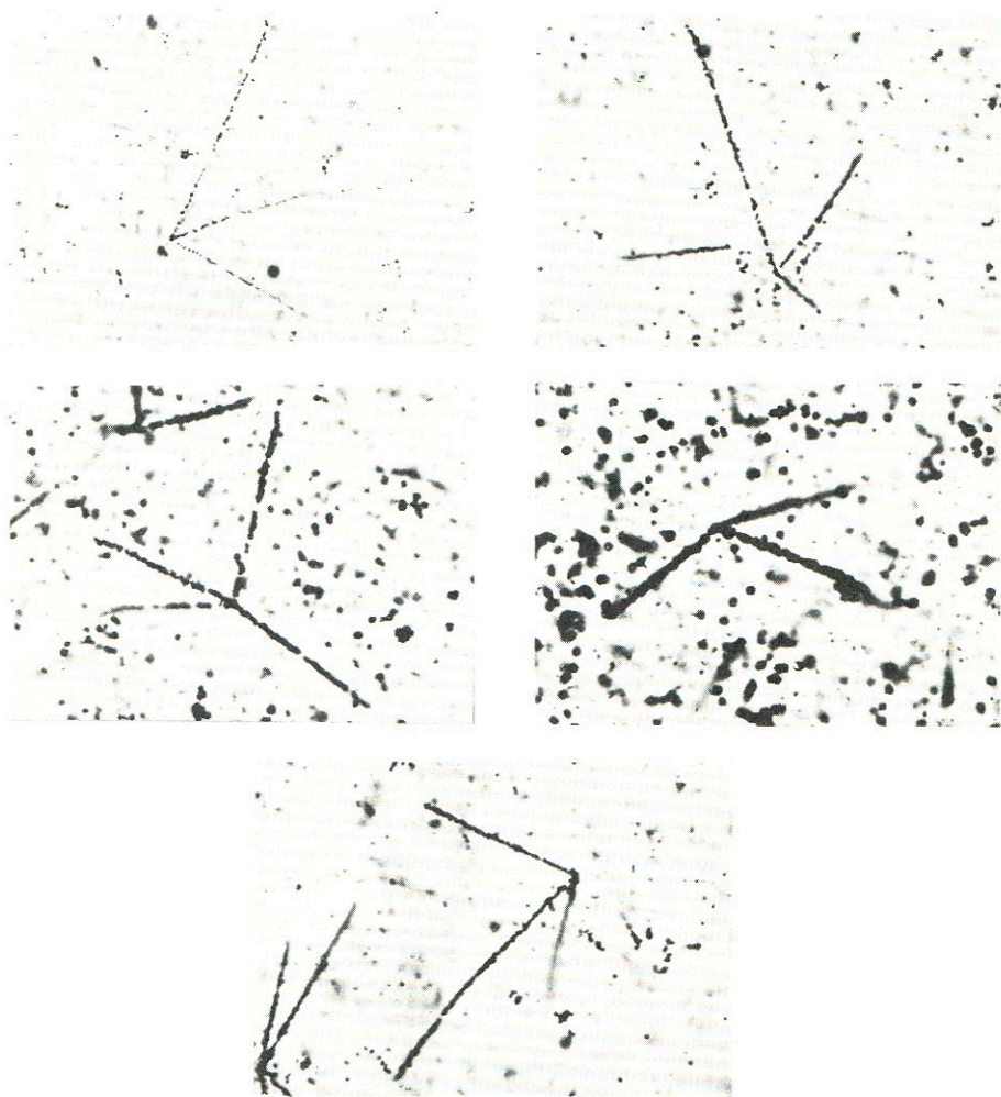
FIG. 2.3.4. Alpha-particle tracks in the same emulsion but reinforced by varying amounts. (Courtesy of P. Cüer.)
