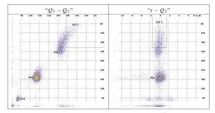
Fig. 7. Correlation diagrams of events registered in a secondary beam  ${}^{12}C + A \rightarrow (Z/A = 7/12) + ...$  at p = 2.0A GeV/c. Left:  $S_3 - S_2$  analyzing counter signals correlation (QDC channels). Right: time-of-flight (ns, faster fragments right) and the  $S_2$  signal correlation.
