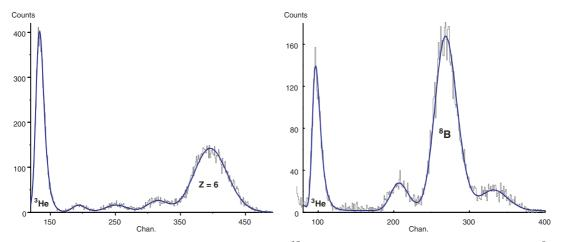
Fig. 5. Secondary beams produced by 2.0 A GeV/c  $^{12}\mathrm{C}$  fragmentation at a beam line tune to the  $^9\mathrm{C}$  fragment rigidity (left) and by 2.0 A GeV/c  $^{10}\mathrm{B}$  at a tune to  $^8\mathrm{B}$  (right).
