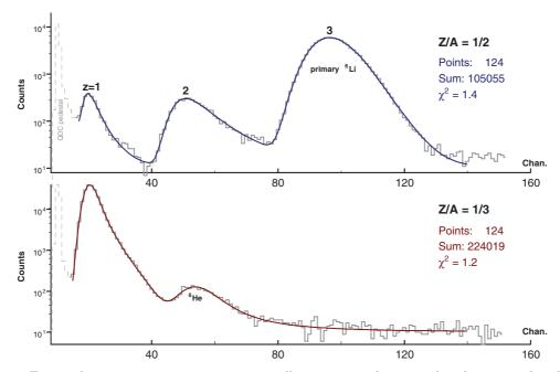
Fig. 4. Energy deposition spectra in a 8 mm scintillator registered in secondary beams produced out of 2.7A GeV/c <sup>6</sup>Li nuclei interaction. Top: at beam line tune to rigidity of fragments with Z/A = 1/2 (scale binding). The predominant peak 3 corresponds to the primary nuclei passed the target without interactions. Bottom: at Z/A = 1/3. Smooth curves are fits of type (3).
