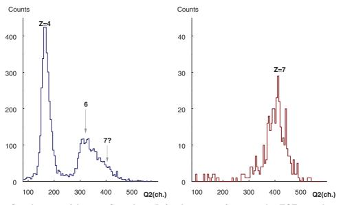
Fig. 8. Signal spectra of the  $5 \text{ mm } S_2$  analyzer. Left: a histogram of events with a TOF cut only vertical solid lines in the right plot of Fig. 7. Right: with an additional low limit cut on the  $S_3$  signal.
