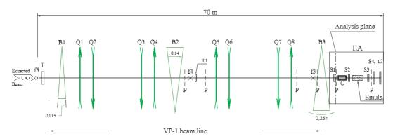
Fig. 3. Optical scheme of the beam line and detectors layout. Dashed marks (P) designate multiwire profilemeters. The  $S_1$  counter of a diagnostic detector assemblage (EA) is placed close to a maximum position (analysis plane) of the beam line resolving function R(z).
