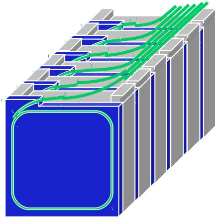
Transverse size  $10 \times 10 \text{ cm}^2$ , length  $\sim 160 \text{ cm}$ , weight  $\sim 120 \text{ kg}$ .
