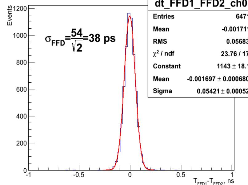
Time difference ( $T_1 - T_2$ ) for 2 FFD modules measured in Dec'12
