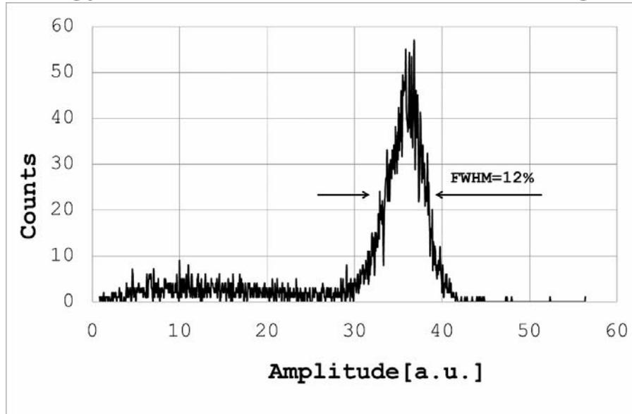
Taking into account position and energy of Compton edge from figure above, energy equivalent of neutron peak measured with lithium glass scintillator in gamma energy scale was found to be 1.7 MeV.
