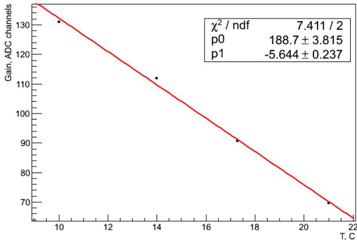
Linear gain drop with temperature
